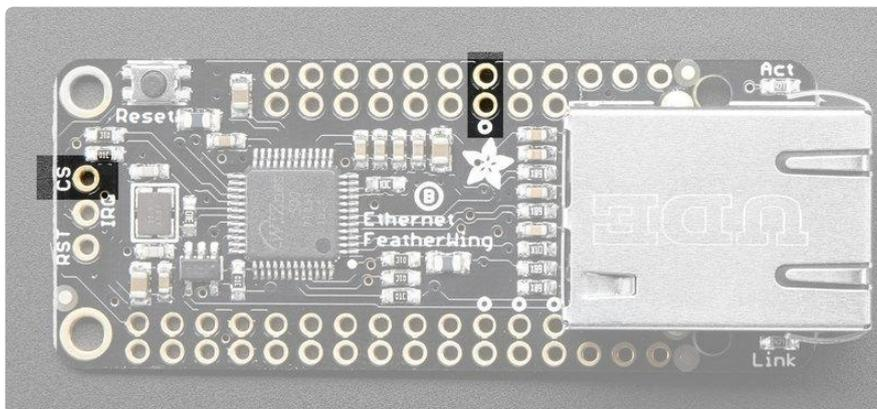
Which is connected to pin #10 on Feather Teensy 3, 32u4, 328p, M4 and M0, pin #15 on ESP8266, and PB4 on WICED.
