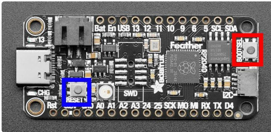
To enter the bootloader, hold down the BOOT/BOOTSEL button (highlighted in red above), and while continuing to hold it (don't let go!), press and release the reset button (highlighted in blue above). Continue to hold the BOOT/BOOTSEL button until the RPI-RP2 drive appears!
