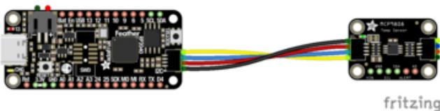
Simply connect the STEMMA QT cable from the STEMMA QT port on your board to the STEMMA QT port on the MCP9808.
