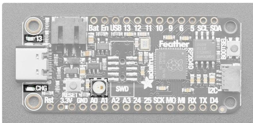
Above the pin labels for A0 and A1 is the status NeoPixel LED. In CircuitPython, the NeoPixel is `board.NEOPIXEL` and the library for it is [here \(\)](#) and in [the bundle \(\)](#). The NeoPixel is powered by the 3.3V power supply but that hasn't shown to make a big difference in brightness or color. In CircuitPython, the LED is used to indicate the runtime status.
