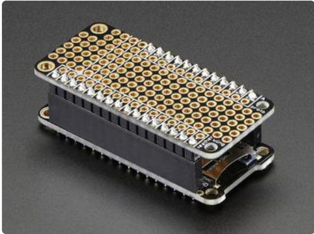
A few Feather boards require access to top-side components like buttons or connectors, making stacking impractical. Sometimes you can stack in the opposite order—FeatherWing underneath—or, if both Feather and Wing require top-side access, place the boards side-by-side with a [FeatherWing Doubler](#) () or [Tripler](#) ().
