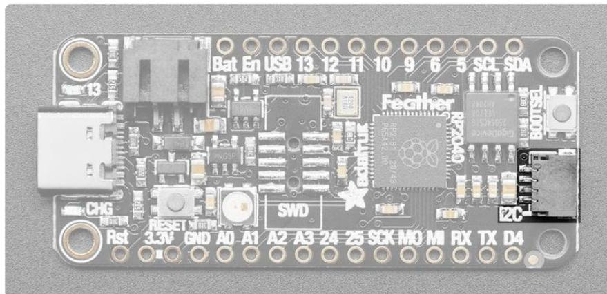
The Feather RP2040 comes with a built in STEMMA QT connector! This means you can connect up [all sorts of I2C sensors and breakouts \(\)](#), no soldering required! This connector uses the SCL and SDA pins for I2C, which ends up being the RP2040's I2C1 peripheral. In CircuitPython, you can use the STEMMA connector with `board.SCL` and `board.SDA`, or `board.STEMMA_I2C()`. In Arduino it is `Wire1`.
