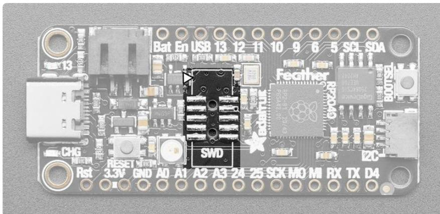
For advanced debugging or to reprogram your Feather RP2040, there is a footprint to solder a 2\*5 pin 0.05" standard SWD header on the board. The image above shows the "pin 1" location by marking it with a triangle. This orientation places the connector key facing towards the end of the board where the USB connector is. This allows you to use something like a [Segger J-Link \(\)](#) and a [1.27mm SWD cable \(\)](#) to connect from your PC to the Feather.
