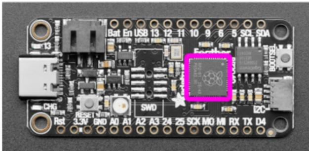
The microcontroller on the Feather RP2040 is located to the right-center of the board, nestled between the Adafruit Feather RP2040 label on the silk.
