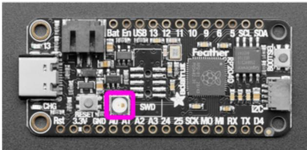
The NeoPixel LED (indicated by the magenta box in the image) is located above the A0 and A1 labels on the silk.
