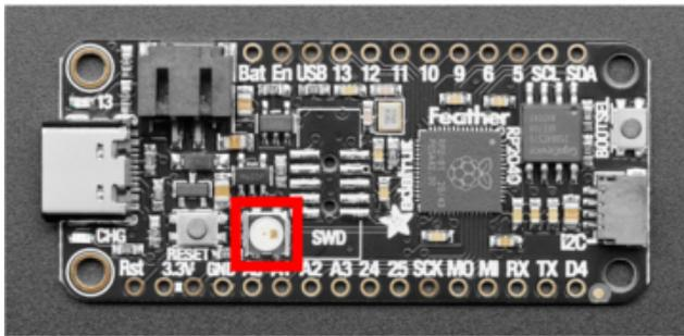
The NeoPixel LED is located between the SWD header and the reset button.
