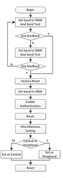
After the initialisation, the Central and Peripheral will do different things, the Central will send message to Peripheral interval and print what received from Peripheral while the Peripheral only responds the Central.
