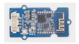
**K2**: During connected status, it could be disconnected by pressing K2 button more than 100ms. During sleep mode, it could be restored through pressing K2 (factory settings) button.
