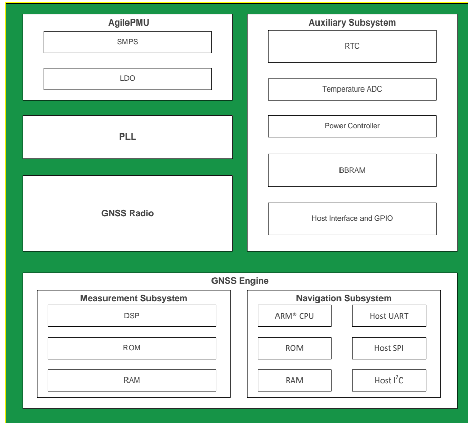
FIGURE 2 – SiRFstarV™ 5e GNSS SoC BLOCK DIAGRAM
