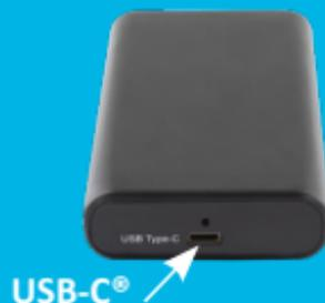
4. Connect the other side of the USB Type-C cable to the USB-C powered device.
