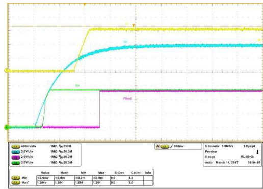
Start up at 23 A Load Ch1:V out , Ch2:PV in , Ch3:P Good , Ch4:V cc
