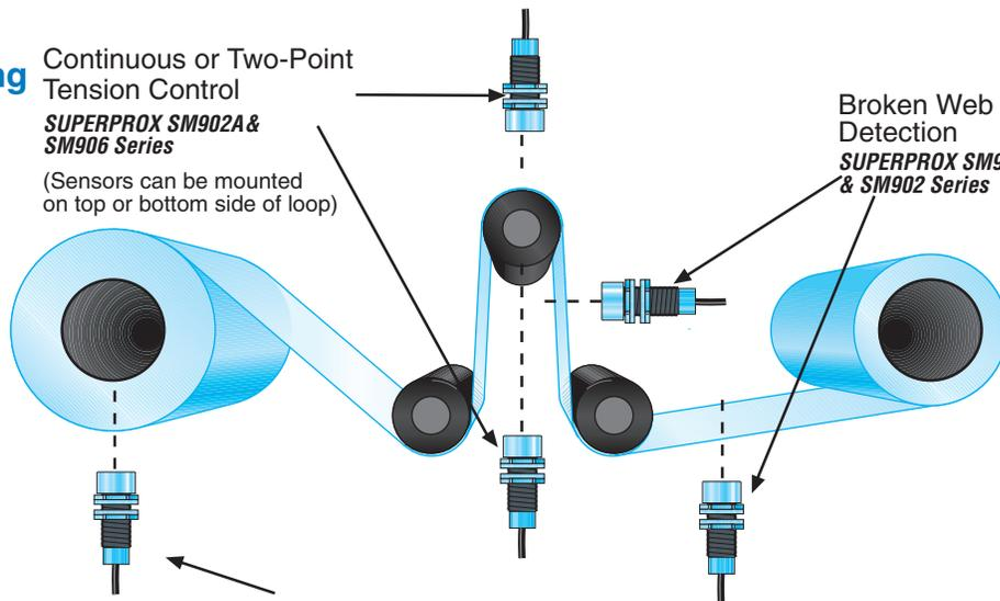
*SUPERPROX SM906* for Roll Diameter Monitoring and
