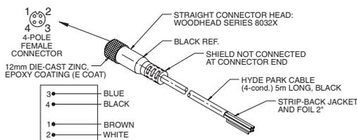
**PB100** In-line accessory push-button for teaching window limits (for Virtu series sensors).
