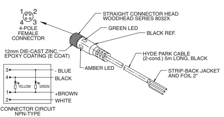
Right-angle, M12 micro, 2-conductor, connector/cable assembly (for SM850 series Transmitters)
