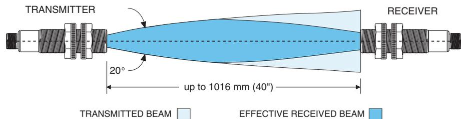
Figure 1, Thru-beam Patterns and Ranges
