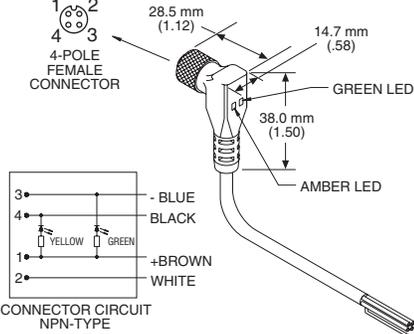
Straight, M12 micro, 4-conductor, connector/cable assembly, 5 m (16'), with built-in LEDs (for SM851 series connector-style Receivers)
