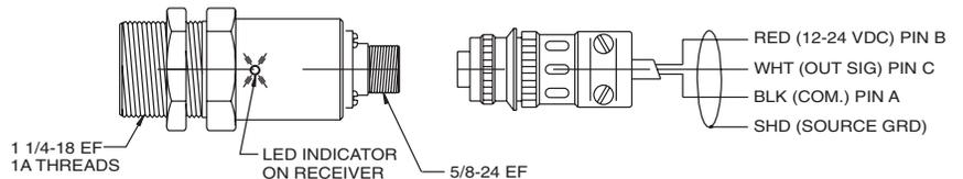
\*\*\* Cable conductor colors vary, dependent upon the sensor model number.
