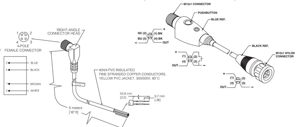
**AC132** Right-angle, M12 micro, 4-conductor, connector/cable assembly, 5 m (16') (for flat-profile connector-style sensors)
