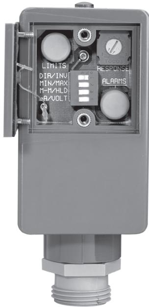
The SUPERPROX® Model SM506A (cable style) and Model SM556A (connector style) ultrasonic, noncontact sensors with a sensing range of 51 mm (2") to 2 meters (79") are readily available. These rugged sensors monitor the distance to an object while generating a proportional analog output relative to two span limits which can be easily set with the push of a button. For applications such as maintaining a constant fill level in a filler machine, the analog
