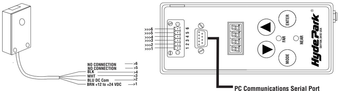
The SC660/SC360/SC390 has reversed outputs; a white-wire NPN and black-wire PNP output
