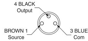
Note: Sensor view-pico connector (pigtail for flat-profile)
