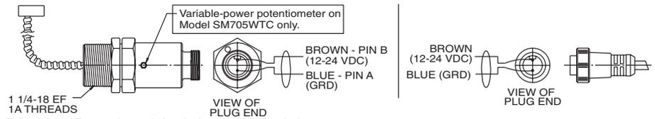
Remote Receiver Models and Model AC108, 7/8-16 mini, 3-conductor, 4 m (12') Mating Connector Cable SM750WTC
