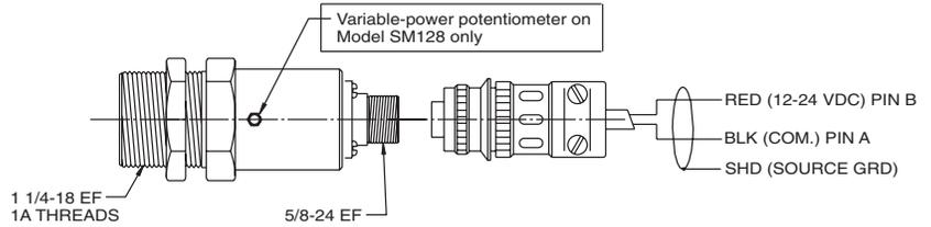
Receiver Models with Model AC150 Amphenol, 3-conductor, 3 m (10') Mating Connector Cable: SM170, 175, 182, 186, 188, 190, 193C, 194, 198C, 199C, 250
