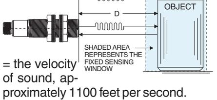
During operation, the calculated distance (D) between the sensor and the object is compared to the distances between the sensor and the fixed window limits. These limits are shown in the illustration as Dwi and Dwo. If D is at or within the fixed window limits, an output change takes place and remains unchanged until the echo either does not return or it returns from outside the fixed window limits.
