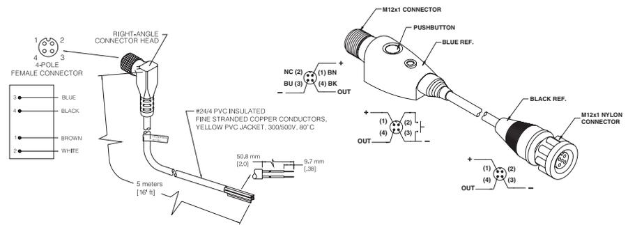
**AC132** Right-angle, M12 micro, 4-conductor, connector/cable assembly, 5 m (16') (for flat-profile connector-style sensors)
