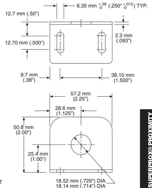
**AC228** Small, right-angle, stainless, mounting bracket (for 18 mm barrel sensors)
