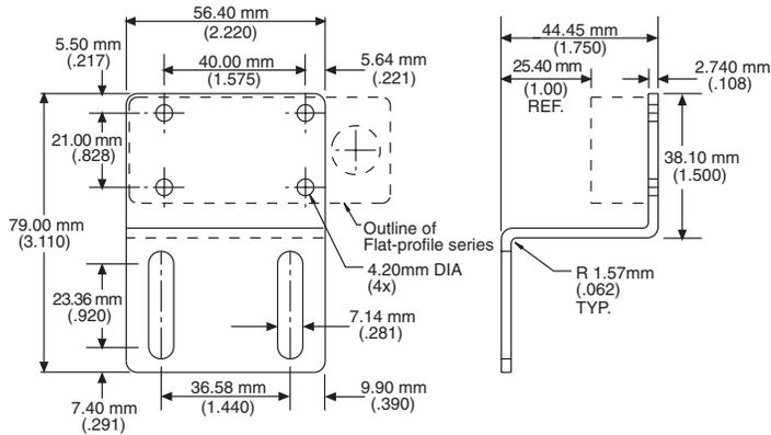
**AC241** Steel/black oxide, 45° angle, label edge mounting bracket used with SUPERPROX SM6X7A-A08-01FP or SM6X7A-A08-11FP flat-profile label sensors
