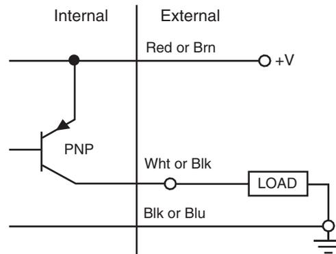
\* Cable conductor colors vary, dependent upon the sensor model number.
