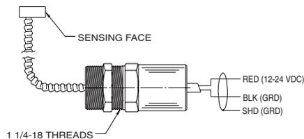
Remote Receiver Models, Standard Cable Length 3 m (10')
