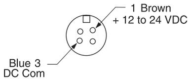
Note: Sensor view-micro connector (pigtail for flat-profile)
