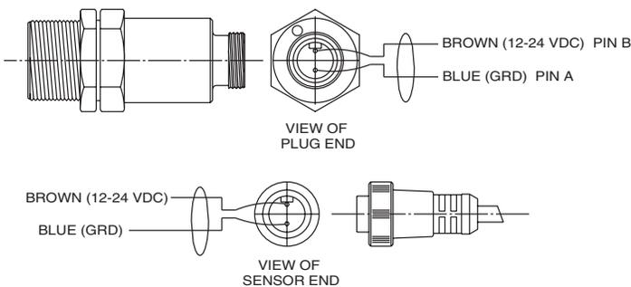
Receiver Models with Model AC108 3-conductor, 7/8-16 mini, 4 m (12') Mating Connector Cable SM186WTC, 190WTC, 250WTC, 252WTC, 256WTC
