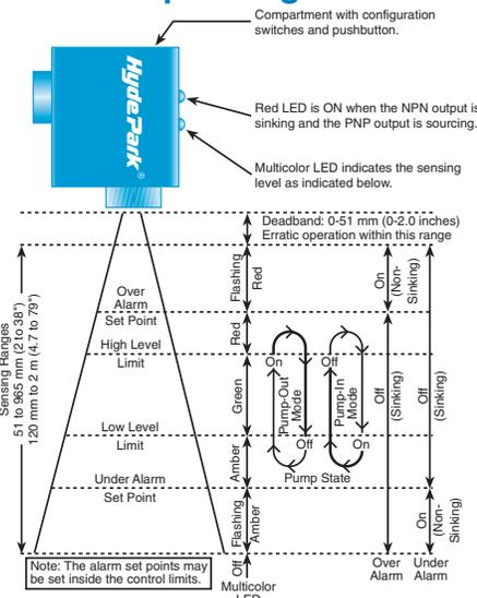
**IMPORTANT:** When either one of the alarm limits is reset for a different level, the other alarm limit must also be re-set.
