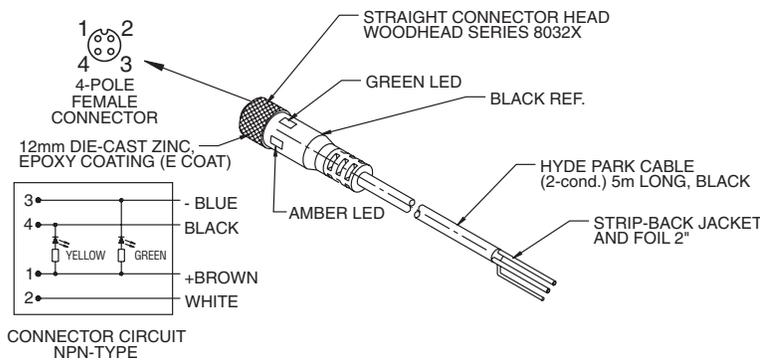
**AC130** Straight, M12 micro, 4-conductor, connector/cable assembly, 5 m (16') (for flat-profile connector-style sensors)
