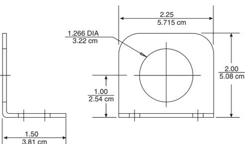
**Model AC213**, Stainless and Teflon, remote sensing probe mounting bracket
