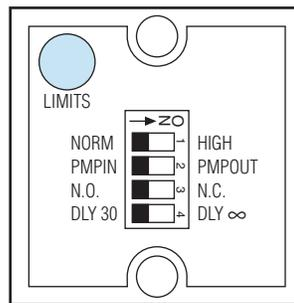
sor output does not change state until the level moves back above the high limit to stop the pumping process.
