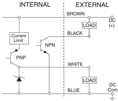
and conductor colors for the Model SM607 series sensors are the same.
