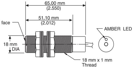
**Barrel Connector Style** (ULTEM® plastic and stainless steel)
