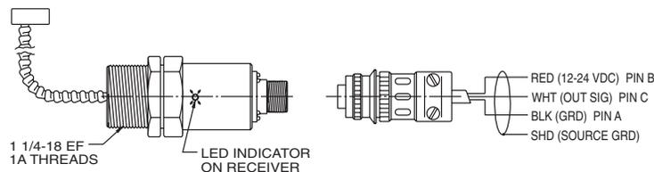
\* Use Belden Cable No. 8423 and No. 9154 to extend receiver and transmitter cable length, respectively. Maximum recommended cable length is 152 m (500").
