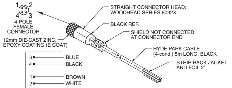
**AC129** Straight, M12 micro, 4-conductor, connector/cable assembly, 5 m (16'), with built-in LEDs (for barrel connector-style sensors)
