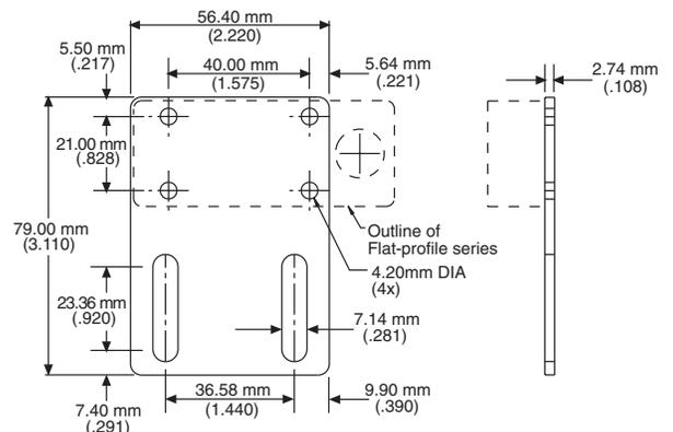
**AC232** S-shaped, stainless mounting bracket (for flat-profile sensors)
