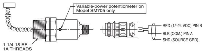
Remote Receiver Models with Model AC150 Amphenol, 3-conductor, 3 m (10') Mating Connector Cable: SM750, 754, 757, 758
