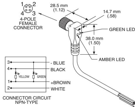
**AC127** Straight, M12 micro, 4-conductor, connector/cable assembly, 5 m (16'), with built-in LEDs (for barrel connector-style sensors)
