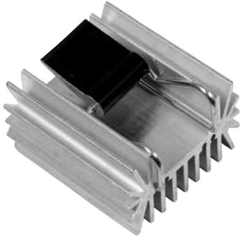
Ohmite's R2 Series (patent pending) heatsink provides a large surface area along with our C Series clipping mechanism to attach to a TO-247 or TO-264 package. The self-aligning features of the clip assure secure attachment and enhanced thermal performance. Because no screws are required for device mounting, additional fins can be added to the rear side of the heatsink for increased total surface area in a more compact space.
