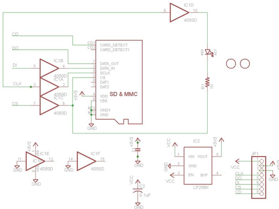
For the level shifter we use the [CD74HC4050 \(https://adafru.it/Boj\)](https://adafru.it/Boj) which has a typical propagation delay of ~10ns
