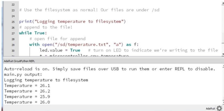
The screenshot shows the Adafruit CircuitPython REPL interface. The top pane displays Python code for logging temperature to an SD card. The bottom pane shows the output of the program, including the message 'Logging temperature to filesystem' and four lines of temperature readings: 26.1, 26.2, 25.9, and 26.0.
