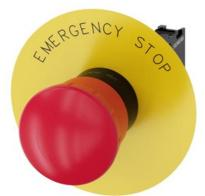
EMERGENCY STOP mushroom pushbutton, 22 mm, round, plastic, red, 40 mm, positive latching, acc. to EN ISO 13850, rotate-to-unlatch, with yellow backing plate, inscription: EMERGENCY STOP, with holder, 1 NC, screw terminal, Z=20-unit packaging
