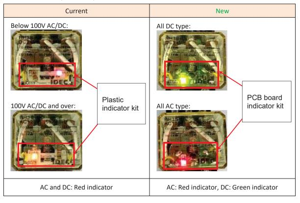
Accordingly, the inner connection will be changed as below.
