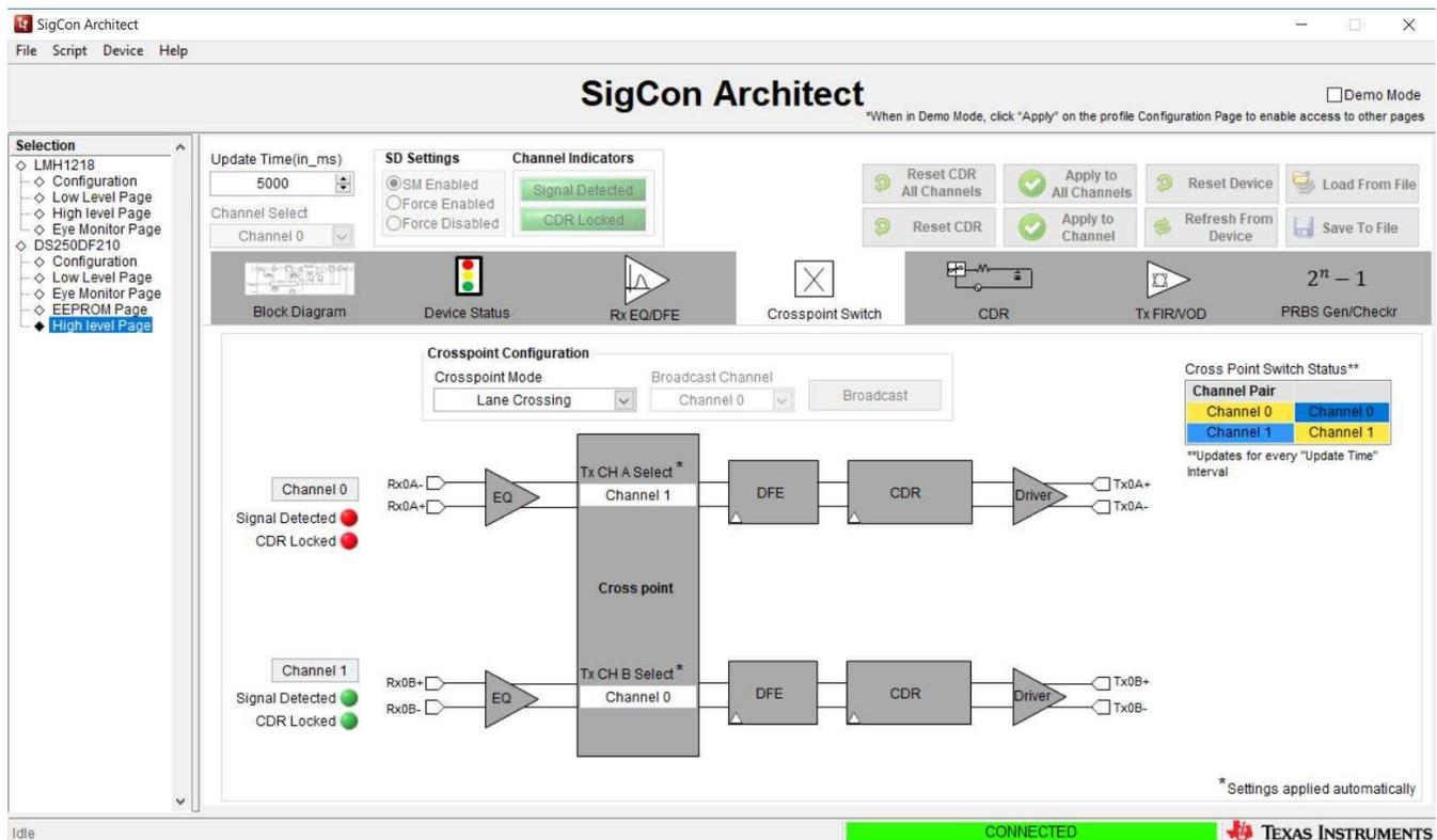
Figure 14. Cross-Point Tab, Lane Crossing Mode Selected
