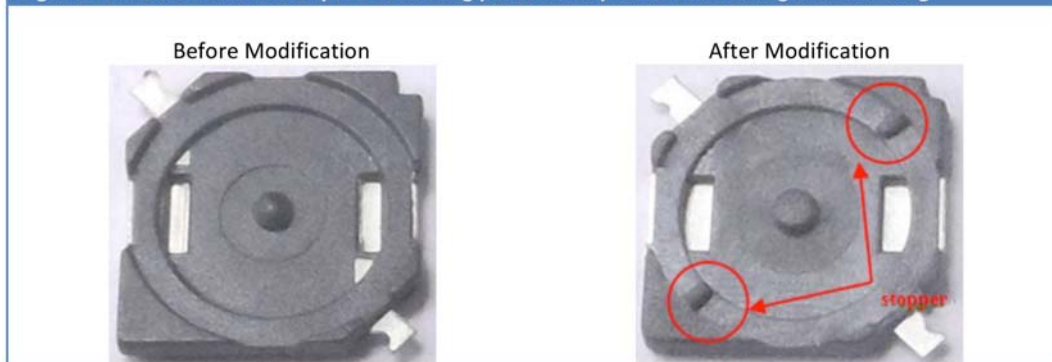
Figure 2. Addition of two bumps to mounting platform to prevent shield ring from rotating.
