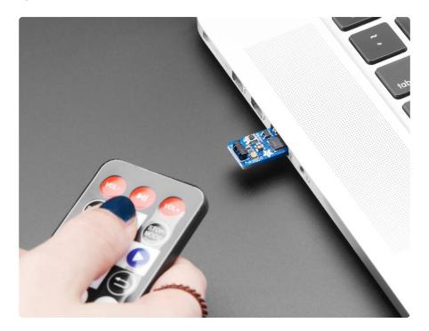
The pIRkey adds an IR remote receiver to any computer, laptop, tablet...any computer or device with a USB port that can use a keyboard. This little board slides into any USB A port, and shows up as an every-day USB keyboard. The onboard ATSAMD21 microcontroller listens for IR remote signals and converts them to keypresses, mouse movements, or even USB serial output.
