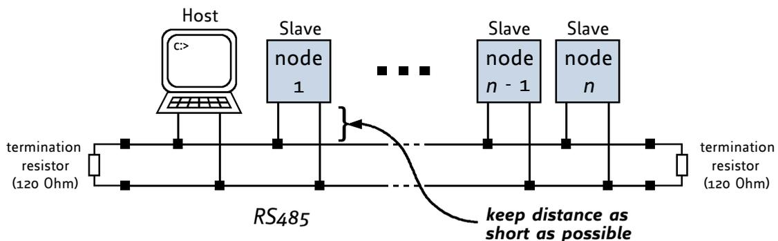
Figure 6: RS485 bus structure with termination resistors
