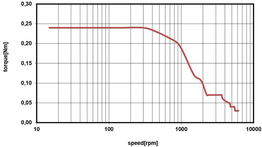
Figure 9: PD42-1-1370 torque vs. velocity 24V / 2A, 256 $\mu$ steps, open-loop
